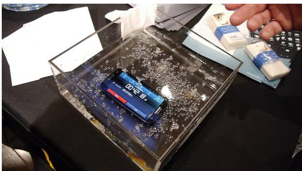
**Figure 5:** P2i water-repellent nanocoating.
